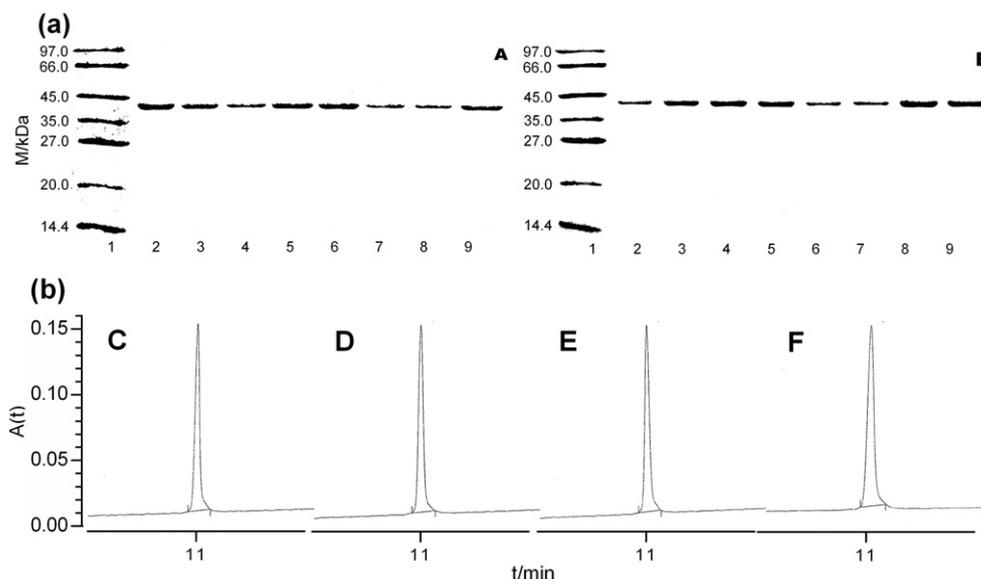
**Fig. 3.** (a) SDS-PAGE lane profiles of CPG2 treated with non-reducing (A) and reducing (B) conditions, after exposure to 24-ns pulses; lanes (1 to 9): molecular mass references M/kDa, and CPG2 exposed to 0, 20, 40, 60, 90, 120, 180 and 240 s of nsEP, respectively. (b) RP-HPLC chromatograms; absorbance  $A(t)$  as a function of retention time  $t/\text{min}$ . Control (C) and CPG2 treated by 8- (D), 16- (E) and 24-ns (F) pulses (with a total exposure time of 240 s); no new peak occurred.
