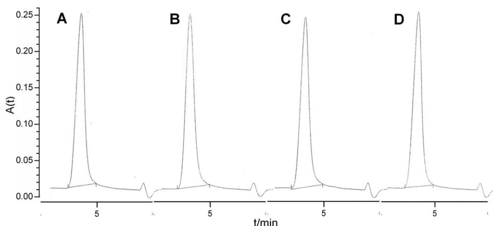
**Fig. 2.** SEC chromatograms; absorbance *A(t)* as a function of retention time *t/min*. Control (A), and CPG2 exposed to 8- (B), 16- (C) and 24-ns (D) pulses. The total exposure time was 240 s. No monomer was detected.
