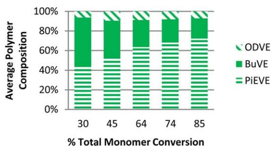
**FIGURE 4** Plot showing average polymer composition versus total monomer conversion for a flow polymerization with an initial monomer charge of 15:4:1 PiEVE:BuVE:ODVE. [Color figure can be viewed in the online issue, which is available at [wileyonlinelibrary.com](http://wileyonlinelibrary.com).]
