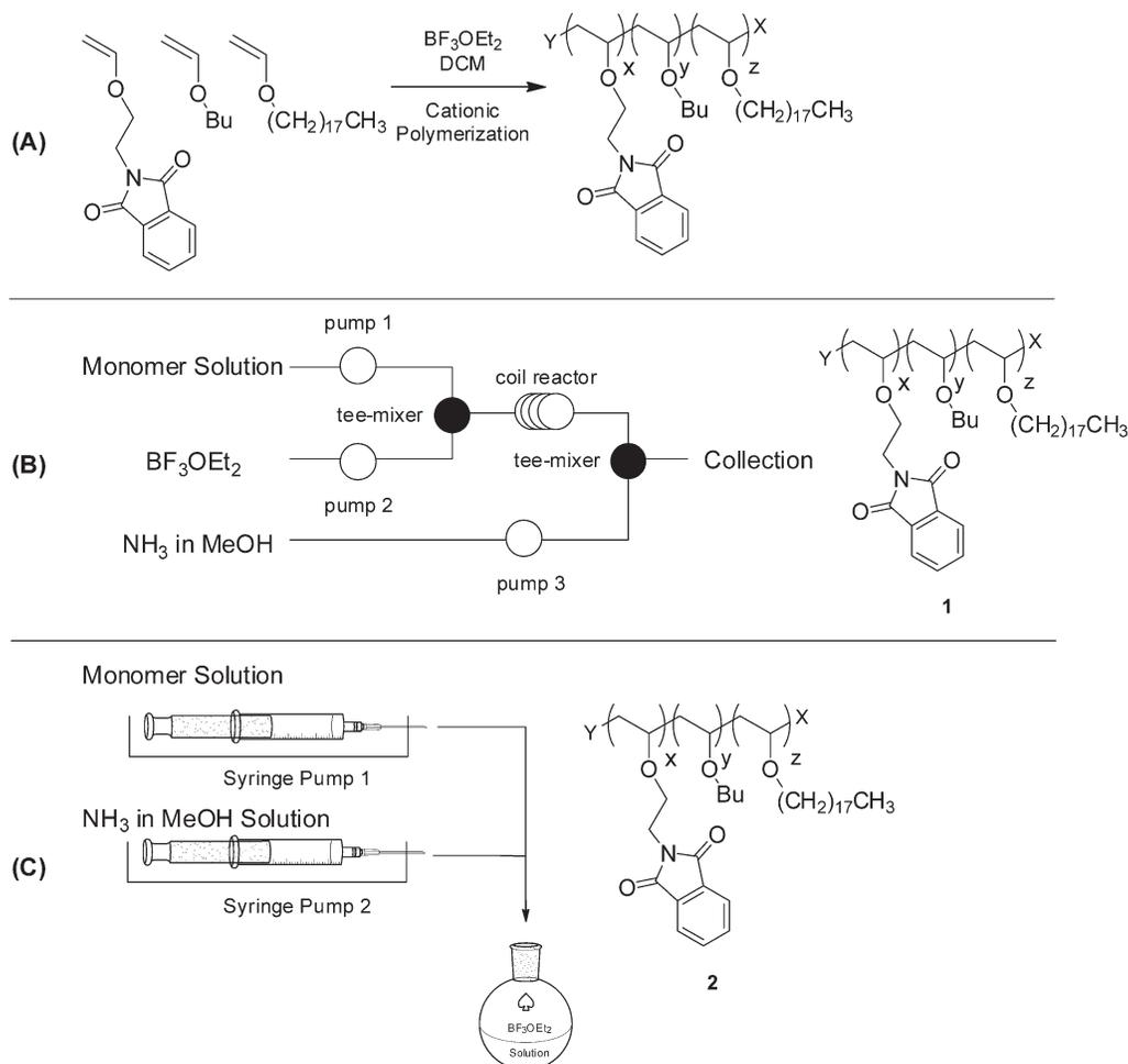
**FIGURE 1** (A) Synthesis of Lewis acid-catalyzed amphiphilic terpolymer. (B) Graphical representation of flow reactor used to produce polymers **1** and **3**. (C) Graphical representation of batch polymerization reaction apparatus used to produce polymer **2**.
