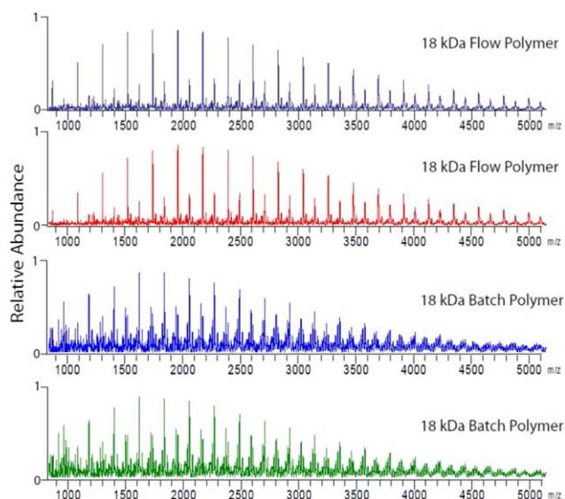
**FIGURE 7** MALDI-TOF comparing protected polymers of the same average molecular weight (18 kDa) generated using the flow. [Color figure can be viewed in the online issue, which is available at [wileyonlinelibrary.com](http://wileyonlinelibrary.com).]
