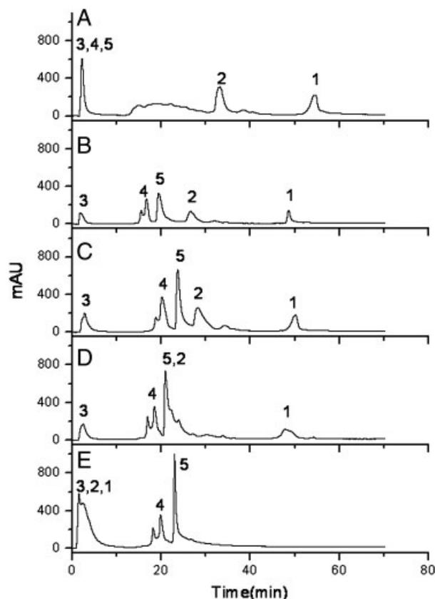
**Figure 2.** Effect of weak anion/cation packing materials ratio w/w on separation of a five-protein mixture with the ratios of WAX and WCX resin as 1:0 (A), 3:1 (B), 1:1 (C), 1:3 (D) and 0:1 (E). Sample: 1,  $\alpha$ -casein; 2, BSA; 3, myoglobin; 4, cytochrome *c* and 5, lysozyme. Injection, 1.5  $\mu$ L. The chromatographic conditions were the same as in Fig. 1C.
