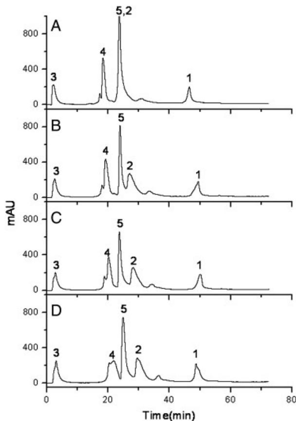
**Figure 1.** Effect of ACN concentration on protein separation using mixed-bed (WAX/WCX = 1:1, w/w; 0.3 mm id  $\times$  100 mm) ion-exchange column. Mobile phase in (A) was A: 10 mM Tris-HCl (pH 8.3); B: A+2 M NaCl (pH 8.3). ACN was added in mobile phases at a concentration of 5% (B), 10% (C) and 20% (D), respectively. Gradient profile: 0–5–75 min, 0–0–70% B. Protein mixture: 1,  $\alpha$ -casein; 2, BSA; 3, myoglobin; 4, cytochrome *c* and 5, lysozyme. Injection, 1.5  $\mu$ L.
