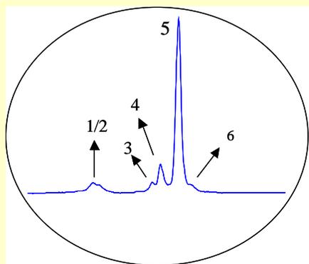
Figure 6 is a typical test chromatogram for a 5  $\mu\text{m}$ , Proteomix SAX-NP column for separation of a mixture of ovalbumin and BSA. High resolution and high selectivity of Proteomix SAX-NP phase can well separate the impurities contained in ovalbumin sample, as well as the BSA dimer from BSA.
