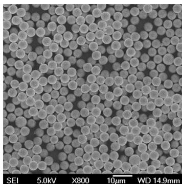
Mono-dispersed Proteomix ion-exchange particles enable uniform column packing bed, which improves separation efficiency.
